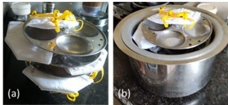
Figure 9: Multiple respirator decontamination possibilities using the boiled hot water technique. (a) 4-stand “idli-cooker” insert used for cycle 6, shown with 4 Venus 4400 respirators. (b) shows the nested vessels (without lids) used for this experiment.
