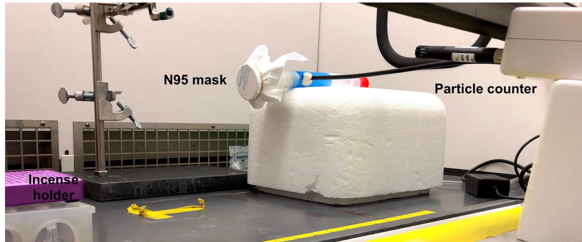
Figure 3: Filtering efficiency test setup to test filter efficiency of a N95 mask using LightHouse handheld particle counter to detect particles of size 0.3 \mu\text{m} - 10 \mu\text{m} produced by burning an incense stick.
