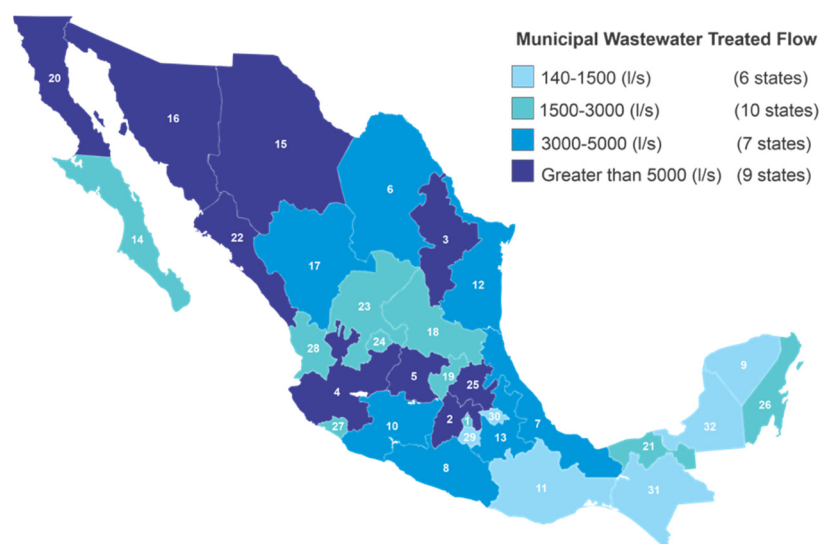
Figure 2. Treated municipal wastewater flow rate by 32 states in Mexico based on CONAGUA data [8] and the National inventory of municipal drinking water and wastewater treatment plants in operation [70].
