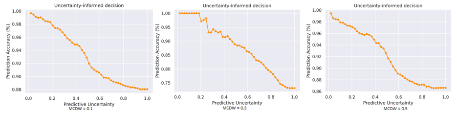
Fig. 6. The classification accuracy as a function of the tolerated normalized model uncertainty
