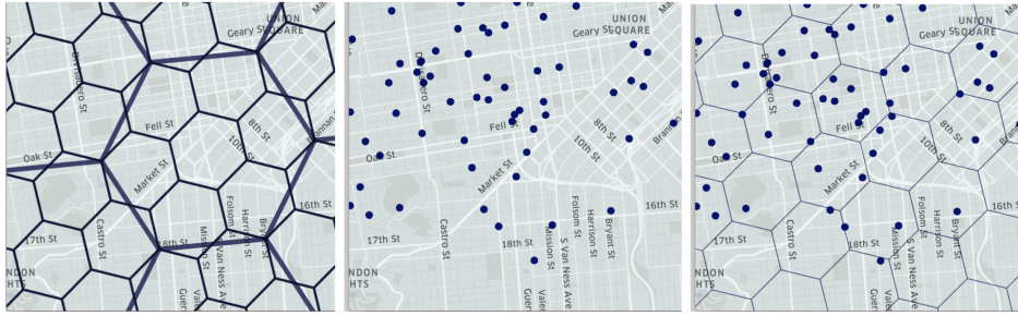
Figure 2: A geographic area partitioned by a hexagonal H3 grid. Points are mapped to an index corresponding to their containing grid cell.
