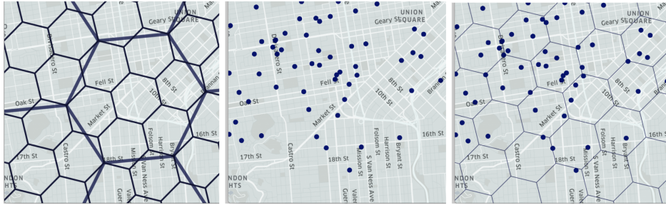
Figure 2: A geographic area partitioned by a hexagonal H3 grid. Points are mapped to an index corresponding to their containing grid cell.
