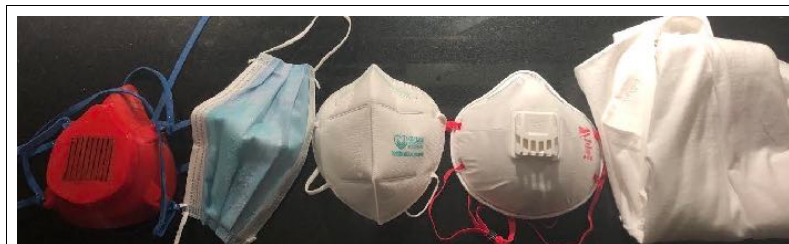
Figure 1: In order from left to right: 3D Printed Reusable N95 Respirator, surgical mask, KN95, N95, cotton cloth.
