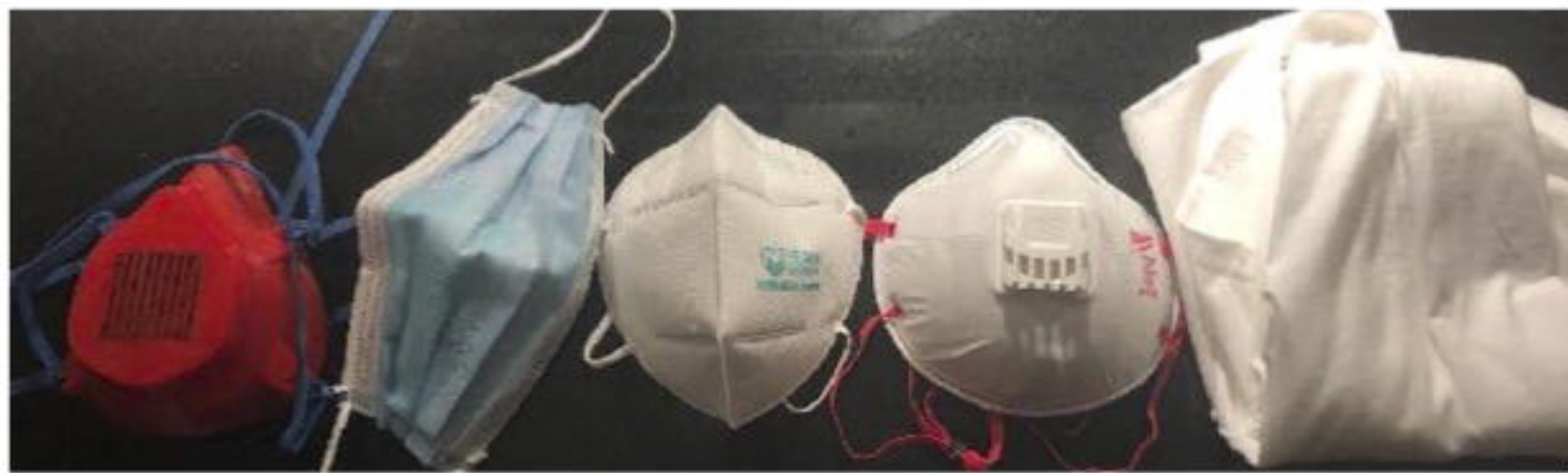
Figure 1: In order from left to right: 3D Printed Reusable N95 Respirator, surgical mask, KN95, N95, cotton cloth.
